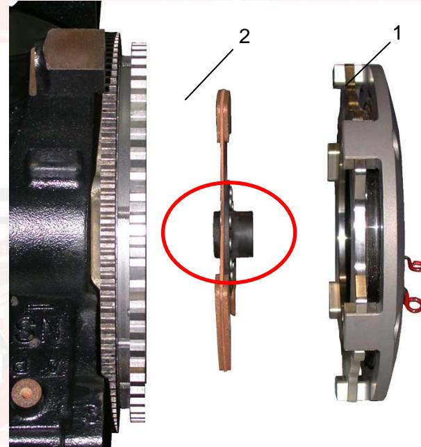
Check the indicator showing whether the clutch assembly and clutch pressure plate are balanced.
